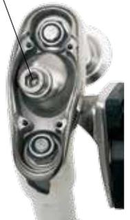
The cars run on Torlon® ball bearings.
