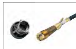
Pull the terminal over the line and fold the core of the line over the wedges. Insert the wedges into the terminal.
